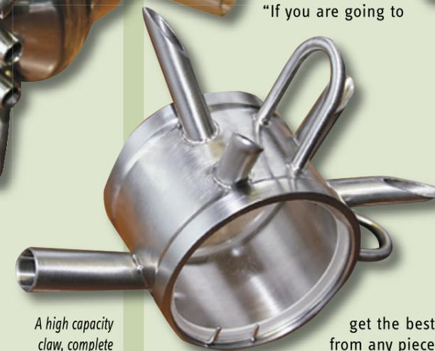
*A high capacity claw, complete with a sight-glass, is recommended for use with high yielding cows to prevent 'flooding'. The air bleed hole is just behind the support loop.*
