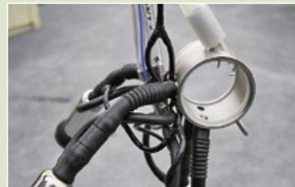
The complete cluster assembled. The small bore dark rubber piping carries the rinsing water for the clusters. About 300ml of water is air-blasted through the liners before the cluster is attached to another cow's udder.
