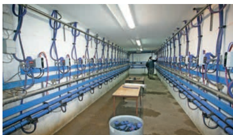
Milk lines and AirWash Plus equipment located in a cellar beneath Hartpury's milking parlour.
